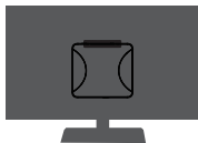
Fix the bracket to the back of the monitor with screws.
